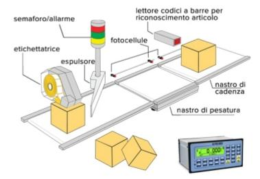
Software version for managing systems that weight packages on a conveyor belt, through static or dynamic weighing and tolerance control. Thanks to the high conversion and acquisition performances and to the advanced filtering functions, it's possible to weigh and memorise an elevated number of packs/min.
