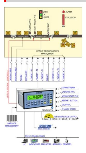
Management of a tolerance control line and static and dynamic weighing of packages on a conveyor belt.
