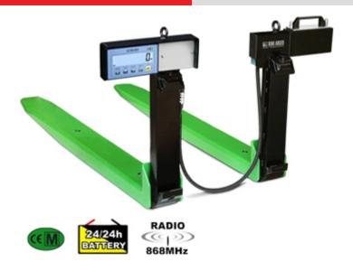
Pair of forks with an integrated weighing system, for lift trucks, easy to use, sturdy, and reliable. Simple and easy to install, these replace the original forks and allow a clear visualisation of the loaded weight. Compatible with any lift truck having a DIN 15173 - FEM fork holder plate, of the IIA or IIIA class (IIB optional). Available in CE-M approved version.
