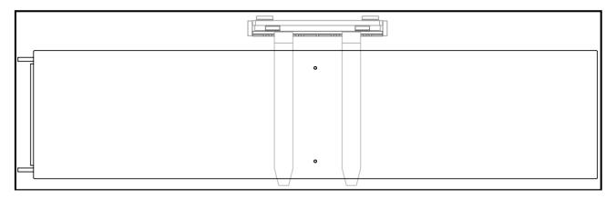
INCORRECT position of the module (bridge) on the forklift truck during the handling procedures.
