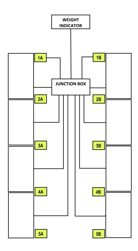
As it can be noticed from the previous image, each weighing bar is fitted with the related labels regarding its position inside the system. These labels are designed to make the installation simple and immediate. The bars and the platforms must be positioned with the labels on their internal side. In the next paragraph more details about these labels are added.
