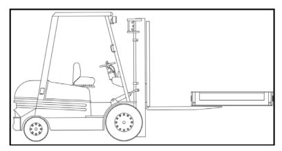
INCORRECT position of the module (bridge) on the forklift truck during the handling procedures.
