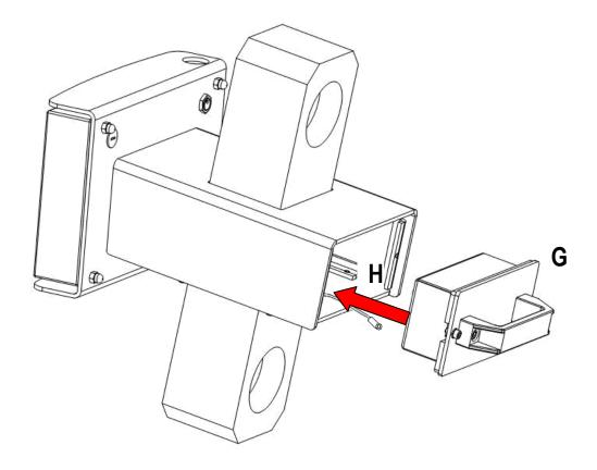
**G:** Are the battery box and the relative way of insertion in the electronic crane scale MCW09.
