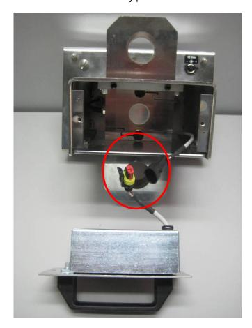
5) Connect the charger to the battery pack by the auto-motive AMP connector.
