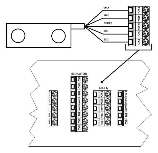
**Note**: with 6 cables load cells, SENSE+ must be short-circuited with EXC+, and SENSE- must be short-circuited with EXC- .
