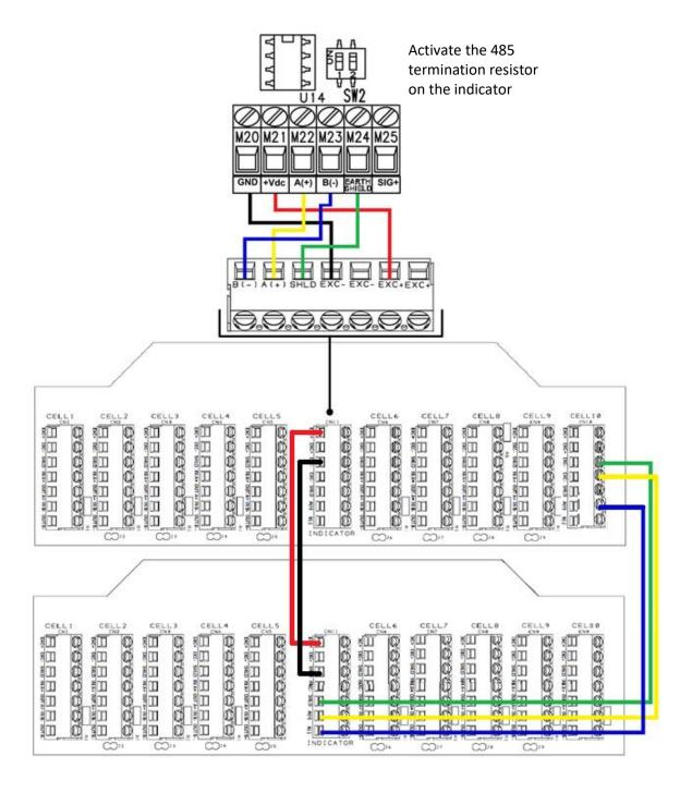
The first board must have all termination jumpers open (including S1).
