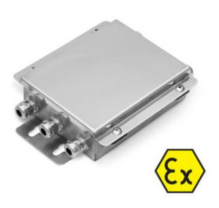
Stainless steel junction box with IP66 protection from water and dust, and fitted with an intrinsically safe electronic board for junction and equalisation of load cells. Terminal boards with screws for easing th connection of the load cells and signal adjustment trimmer, for an accurate and reliable equalisation. Marking: ATEX II 2G Ex ib IIC T6 Gb for gases.
