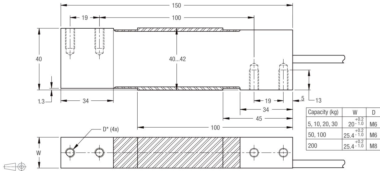
Mounting bolts up to 100 kg: M6 8.8 / torque 10 Nm; for 200 kg: M8 8.8 / torque 25 Nm. Torque values assume oiled threads.
