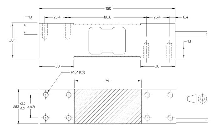
Mounting bolts M6 8.8; torque 10 Nm. Torque value assumes oiled threads.
