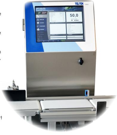
The C80 checkweigher is easy to clean with quick belt release (accessory) and incorporates an open stainless steel and corrosion free load cell, guaranteeing trouble-free weighing.
