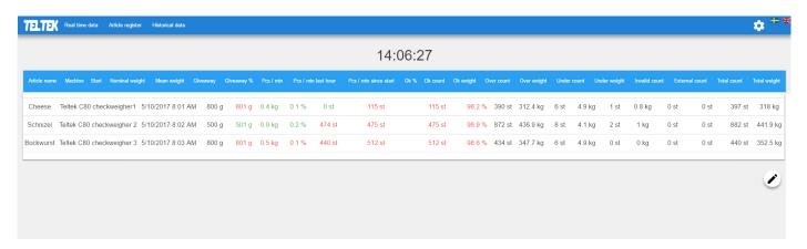
Teltek InControl can be accessed from your regular web browser. You can connect from your PC, your tablet or your smartphone. No need for installation of special software for client use. Teltek InControl is an SQL based production monitoring software.
