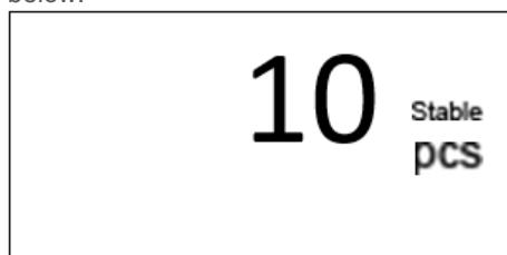
Take off the samples on the pan. The sampling operation is finished. Then the balance can be used for counting.
