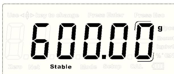
If the Capacity of the balance is 300.00, 1200.0, 1500.0 and 3000.0g, the last digit will be blank in normal weighing mode only if the EXT.D key is pressed to extend the display.
