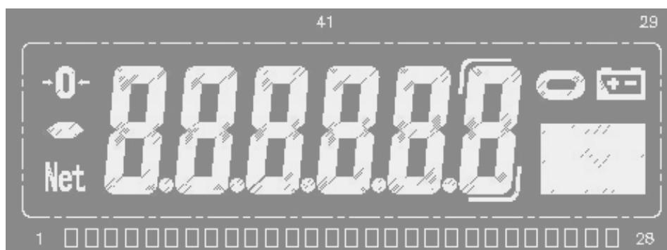
If the Capacity of the balance is 600.0g, the last digit will be the auxiliary display digit (a symbol indicating the digit):
