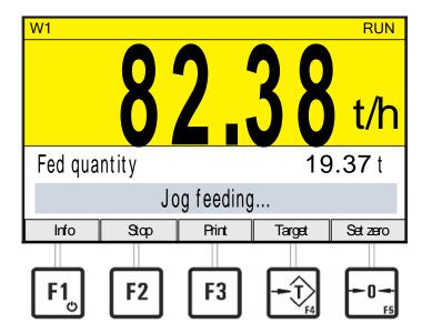
After expiry of the jog time the external output 'Pre-signal' and/or the corresponding bit on the fieldbus are reset and the stop delay time is started anew.
