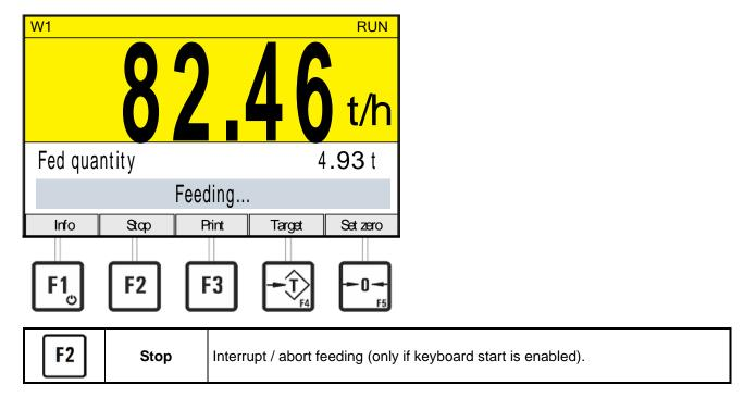
Feeding can be continued with the rising edge of the external start/stop signal or the 'Run' bit of the fieldbus data word. If keyboard start is enabled in the configuration, feeding can also be continued with the F2-key 'Resume'. An interrupted feeding cycle can be aborted with the F5-key 'Abort' or the corresponding bit of the fieldbus communication.
