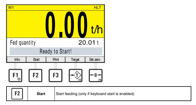
With the start of feeding the fed quantity is reset to zero.
