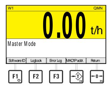
F1<sub>o</sub> Software ID Show version No. of approved scale software and its identification No.
