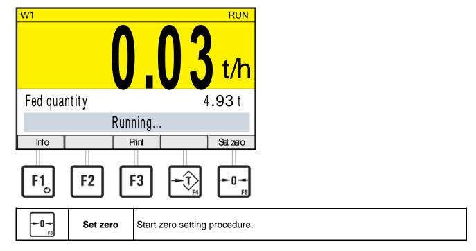
During the zero setting procedure the external output 'Setting zero' and/or the corresponding bit on the fieldbus is set. If the permissible zero setting range is left during zero setting the procedure is automatically aborted. Zero setting must then be triggered anew.
