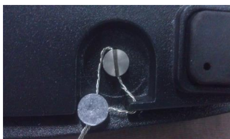
Locked with Wire Seal
