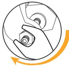
g. Tighten the locknut, to lock the adjustment screw.
