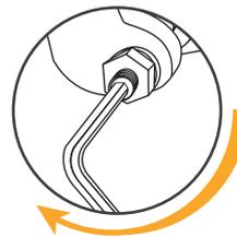
e. Slowly turn the adjustment screw clockwise until the forks start moving downwards.
