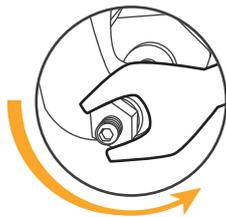
d. Unscrew the locknut, to unlock the adjustment screw.
